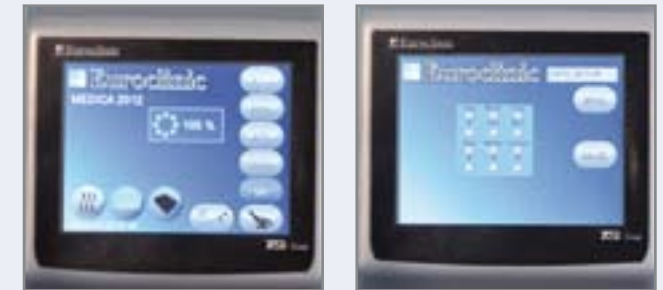
Screen shot - 1. Visualization and control of the light intensity for LED light source - 2. Language selection (Italian, English, French, or any national language on request) and date selection
